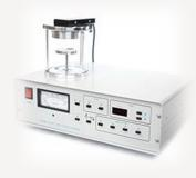
The automatic sputter coater deposits a fine gold layer onto samples using high-vacuum sputtering. Argon plasma ablates gold atoms from a target, depositing them evenly on the sample. Metallisation is essential to render biological samples conductive, reduce charging, and preserve ultrastructural detail during SEM analysis.
