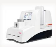
The Leica EM CPD300 is an automated critical point dryer used for SEM sample preparation. This technique preserves the three-dimensional morphology of samples by avoiding the surface tension artefacts associated with traditional drying methods. The system uses carbon dioxide as a transitional fluid and gently removes solvents at their critical point. Automation ensures reproducibility and minimises error.
